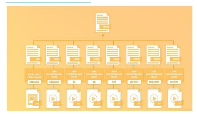
HLS streaming is a truly adaptive bitrate technology. When video is encoded to HLS multiple files are created for different bandwidths and different resolutions. The files are encoded using the mpg2\_ts codec. The streams are mapped to the client in real time using an .M3u8 index file based on screen size and available bandwidth.
