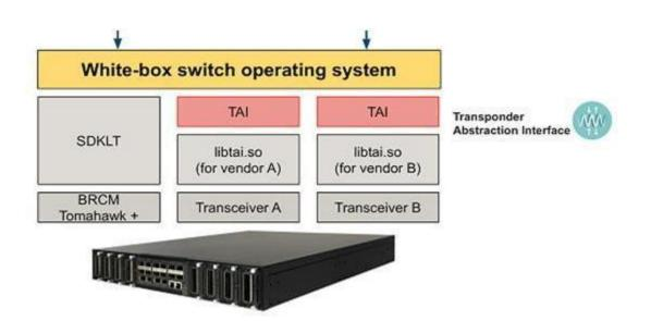
The TAI layer provides generic API's to switch operating system to manage the optical coherent- devices. The switch operating system uses the TAI abstraction layer to talk to vendor-specific driver code (libtai-dco.so) to program the underlying coherent-device. As part of this integration, we also designed and developed the libtai.so driver for DCO optical CFP2 module.
