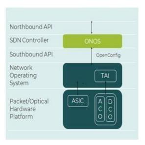
ODTN enables end-to-end orchestration leveraging the Open Network Operating System SDN controller (ONOS) to provide control, management and provisioning of networks and equipment. The open design enables ONOS to configure the optical modules using ONOS data- models. These OpenConfig specific data-models were developed as part of this project.
