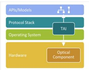
As part of this project, we integrated open-source TAI library in to NOS and developed TAI complaint vendor specific driver modules, the architecture of which is as shown below.
